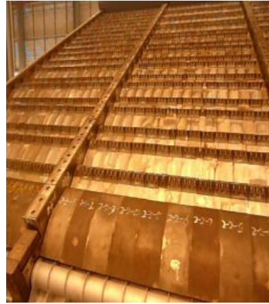
Figure 10 Schematic Representation of a Reciprocating Grate Facility:
