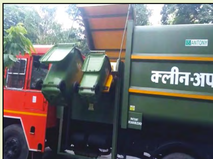
Compactor with separate chamber for collection of Dry waste and E waste
