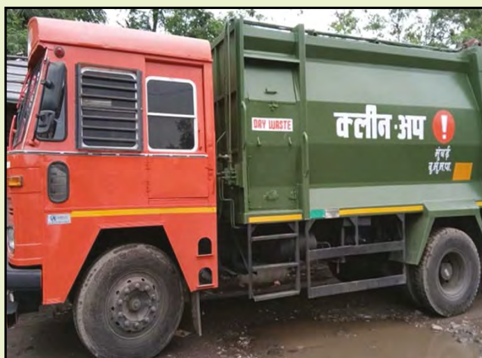
Compactor with Additional Chamber of Dry Waste Garbage
